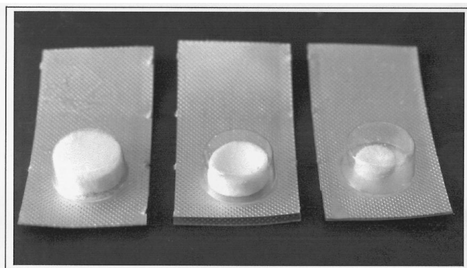
Figure 3. Formulation A packed in PVC/aluminum blister packs at time T_0 and after storage for 1 month and 3 months at 85% relative humidity.
